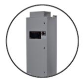
HPS TruWAVE monitors the load current and very quickly responds to the power system distortion as it develops. A corrective current is injected to effectively cancel out the harmonics required from the upstream power source. The result is a harmonic load on the power system that is acceptable, with more balanced current and voltage waveforms.
